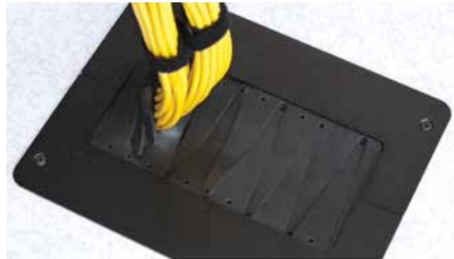
Non-permeable material allows maximum pressure to be maintained in the sub-floor plenum when cables are installed; minimizing bypass airflow.
