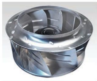
Optional EC Fan Technology available in selected Compu-Aire Inc. systems. The evaporator sections are configured for draw-thru air pattern to provide uniform air flow over the coil face area. Each fan is a cassette type complete with a variable speed high efficiency EC motor directly driven by the controller with 0-10 VDC output for precise air flow volume control.
