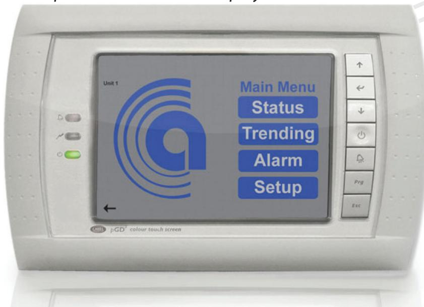
Included are various animated icons and non-proportional fonts in Unicode format and trend graphs. The touch screen display functions simplify setting the control parameters, allowing the customer easy access to the System 2200+ series controller.
